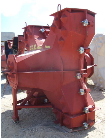
PRODUCTION OF CONCRETE HEXAPOD
