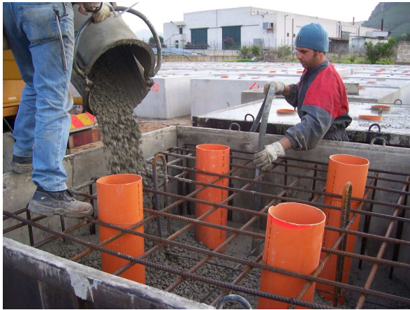
PRODUCTION OF CONCRETE CUBIC BLOKS
