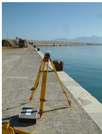
POSITIONING OF GPS RECEIVER ON DATUM POINT
